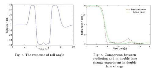
Figure 6 shows the test data of roll angle under the condition of double lane change. And the comparison of the roll angle in next period between the value predicted by BP neural network and the value acquired by experiments under the same conditions are shown in Figure 7. As Figure 7 shown, the predicted value of the roll angle is consistent with the actual data. It can be seen that the motion parameters in the future time can be predict effectively based on HMM and ANN.
