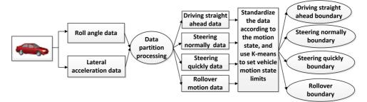
Fig. 1. Preprocessing process of acquisition data
