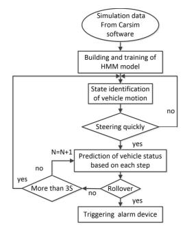
Fig. 3. Flow diagram of rollover warning
